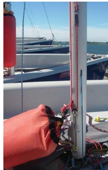
With the older Proctor masts the front part of the halyard can be passed between the adjuster and the spreader bracket, reducing the impact on mast bend. The later spreaders have a hole in a similar position.
