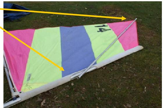
5. The whole rig can now be picked up and placed in mast step in the Optimist.
