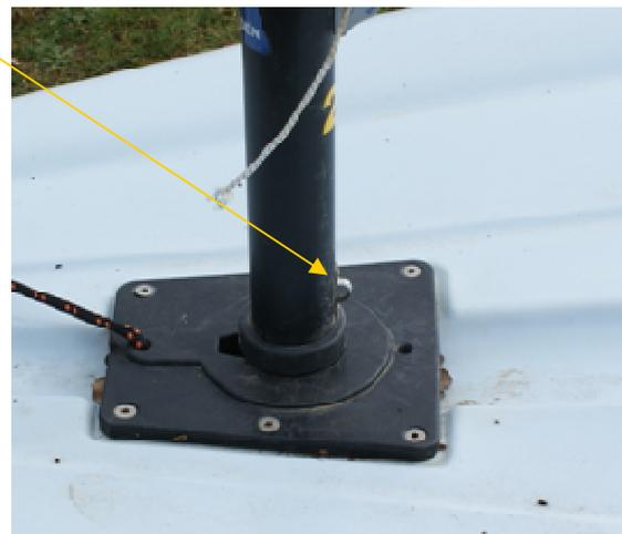
4. Attach boom to mast above gooseneck
